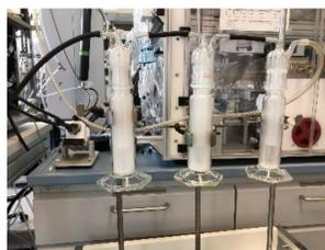
**Figure 1:** row of 3 impingers to trap the different aerosols
