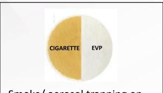
Smoke/ aerosol trapping on Cambridge filter pads
