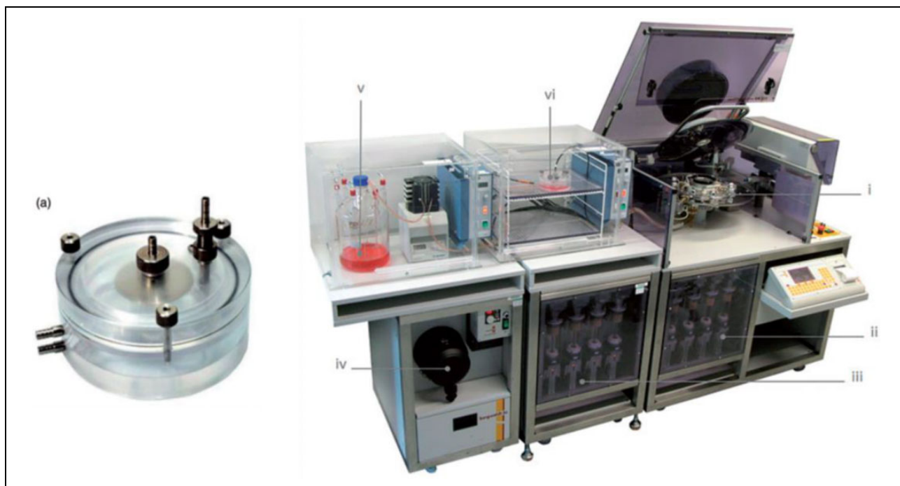
Figure 1. British American Tobacco's standard exposure chamber and the Borgwaldt RM20S smoking machine. (i) Cigarette smoke generator. (ii) Original four-syringe system. (iii) Four-syringe extension. (iv) Air-flow controller. (v) Cell culture media maintained at 37°C. (a) British American Tobacco's exposure chamber housed at 37°C, attached to the smoke diluter and culture medium reservoir. 20
